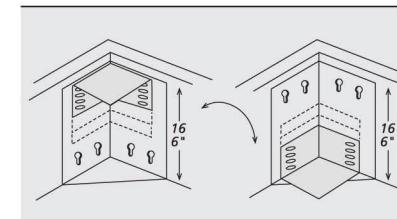
A special metal support allows to place the slats in different positions from 2 cm - 3/4" to 18 cm - 7" from the edge of the bed base.
