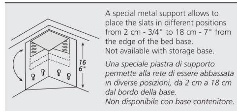
A special metal support allows to place the slats in different positions from 2 cm - 3/4" to 18 cm - 7" from the edge of the bed base.
