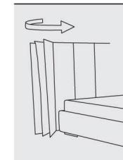
Headboard with mechanism allows movement of side panels in different positions.
